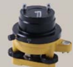
Tribrach optical plummet alignment
